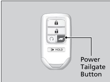
Press the power tailgate button for more than one second to operate when the power mode is in VEHICLE OFF (LOCK).
