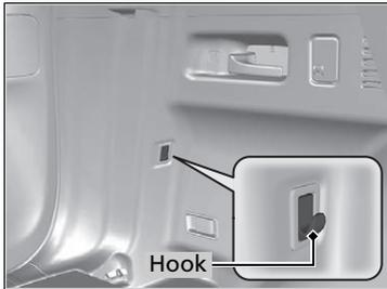
The cargo hooks on the driver's side of the cargo area can be used to hang a light items.
