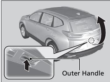
When all the doors are unlocked or press the tailgate unlock button on the remote transmitter, the tailgate is unlocked. Press the tailgate release button and lift open the tailgate.
