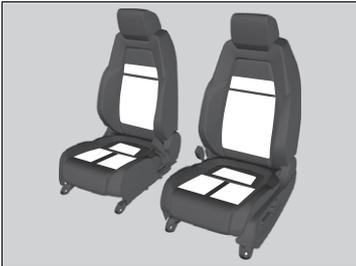
The power mode is in ON to use the seat heaters. The HI setting heats the seats faster than the LO setting.
