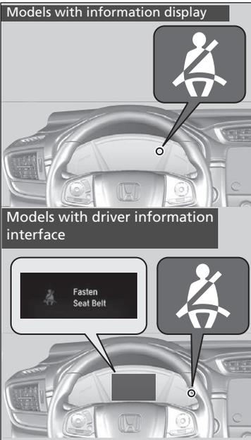
The seat belt system includes an indicator on the instrument panel to remind the driver or a front passenger to fasten their seat belts.
