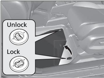
The driver's floor mat hooks over floor anchors, which keep them from sliding forward. To remove a mat for cleaning, turn the anchor knobs to the unlock position. When reinstalling the mat after cleaning, turn the knobs to the lock position.
