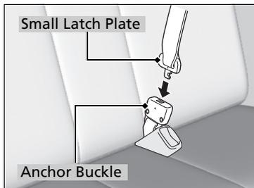
2. Line up the triangle marks on the small latch plate and anchor buckle. Make sure the seat belt is not twisted. Attach the belt to the anchor buckle.
