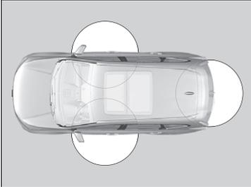
When you carry the smart entry remote, you can lock/unlock the doors and open the tailgate.
