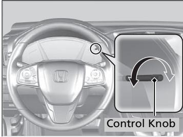
With the parking lights are turned on and the ignition switch is in ON
