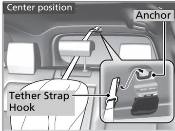
5. Route the tether strap through the head restraint legs. Make sure the strap is not twisted.
