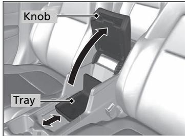
To open, pull the knob. You can change the position of the tray by sliding it forward or back.
