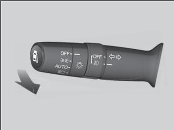
Disable or re-enable the system when the vehicle is parked and the power mode is in ON and the light switch is in the **AUTO** position.
