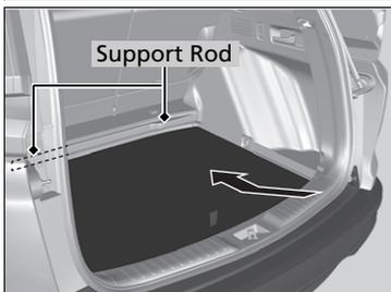
3. Push the far end of the lid down to the bottom under the support rod, then lower the other end.
