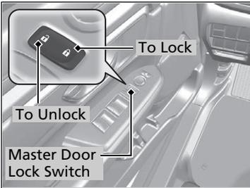
Press the master door lock switch in as shown to lock or unlock all doors and the tailgate.
