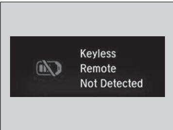
Warning buzzers may sound from inside or/ and outside the vehicle to remind you that the smart entry remote is out of the vehicle. If the buzzer continues even after the remote is put back inside, place it within its operational range.
