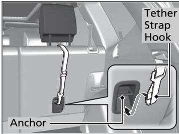
■ **Using an outer anchor**
