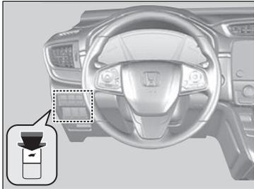
To open or close the power tailgate, press the power tailgate button for about one second. Some exterior lights flash and the beeper sounds.
