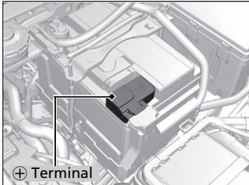
1. Open the terminal cover on your vehicle's battery positive ⊕ terminal.
