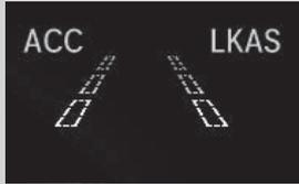
When the LKAS is suspended, the lane lines on the driver information interface change to contour lines.
