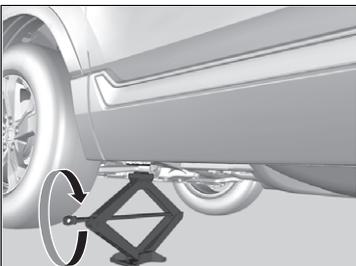
2. Turn the end bracket clockwise (as shown in image) until the top of the jack contacts the jacking point.
