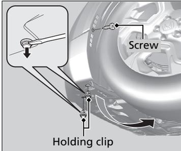
1. Remove the screw using a Phillips-head screwdriver and remove the holding clips using a flat-tip screwdriver.
