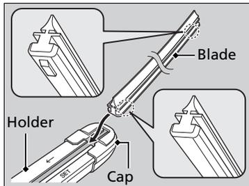
3. Pull the end of the wiper blade to the direction of the arrow in the image until it unfastens from the holder's end cap.
