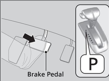
2. Check that the shift lever is in **P**, then depress the brake pedal.
