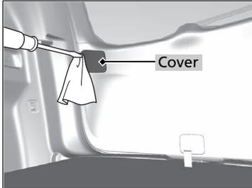
2. Remove the cover by prying on the edge using a flat-tip screwdriver.
