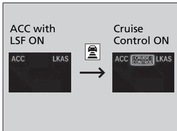
Press and hold the
