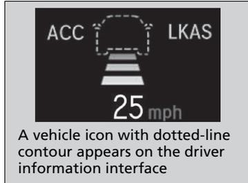
Your vehicle maintains the set speed without having to keep your foot on the brake or accelerator pedal. If there previously was a vehicle detected ahead that kept your vehicle from traveling at the set speed, ACC with LSF accelerates your vehicle to the set speed, and then maintains it.
