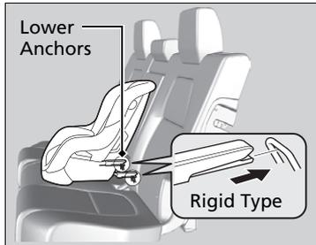
2. Place the child seat on the vehicle seat, then attach the child seat to the lower anchors according to the instructions that came with the child seat.
