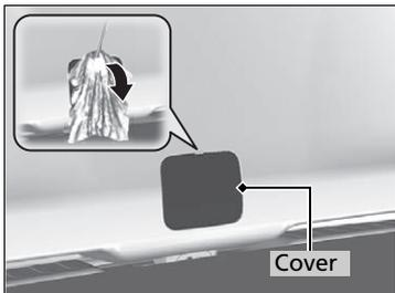
1. Use a flat-tip screwdriver and remove the cover on the inside of the tailgate.
