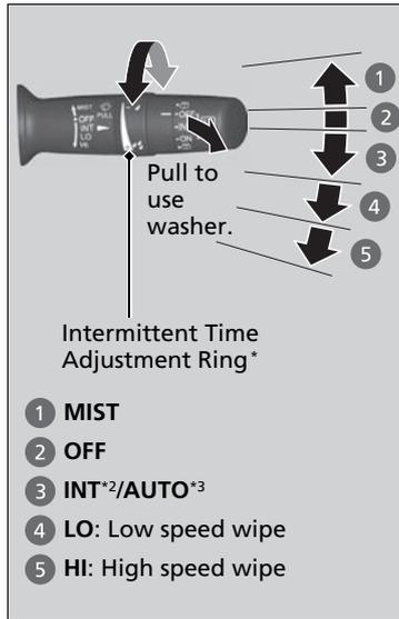
The windshield wipers and washers can be used when the ignition switch is in ON \*<sup>1</sup>.
