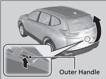
If you press the outer handle of the tailgate for no longer than one second, the tailgate opens automatically.
