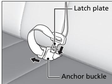
1. Store the center seat belt first. Insert the latch plate into the slot on the side of the anchor buckle.
