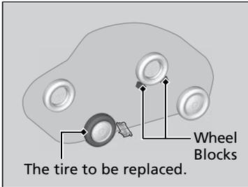
5. Place a wheel block or rock in the front and rear of the wheel diagonal to the flat tire.
