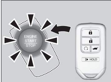
1. Touch the center of the **ENGINE START/STOP** button with the **H** logo on the smart entry remote while the **ENGINE START/STOP** button is flashing.
