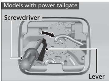
2. To open the tailgate, push the tailgate while pushing the lever to the right using a flat-tip screw driver.
