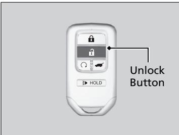
**To open:** Press the unlock button, and then within 10 seconds, press it again and keep it pressed. If the windows and moonroof\* or Panoramic Roof\*<sup>1</sup> stop midway, repeat the procedure.
