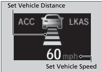
When ACC with LSF starts operating, the vehicle icon, distance bars and set speed appear on the driver information interface.
