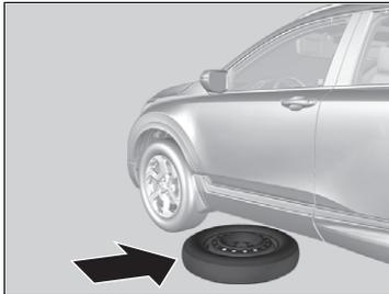
6. Place the compact spare tire under the vehicle body (wheel side up) near the tire that needs to be replaced.
