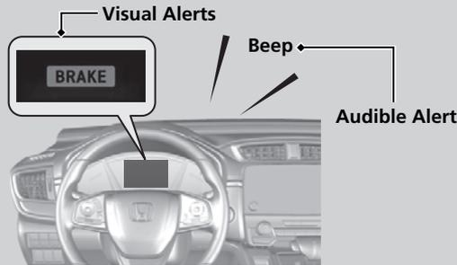
At system's earliest collision alert stage, you can change the distance (**Long/Normal/Short**) between vehicles at which alerts will come on through multi-information display setting options.
