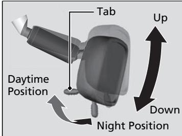
Flip the tab to switch the position. The night position will help reduce the glare from headlights behind you when driving after dark.
