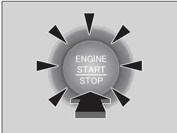
2. Depress the brake pedal and press the **ENGINE START/STOP** button within 10 seconds after the beeper sounds and the indicator changes from flashing to on.
