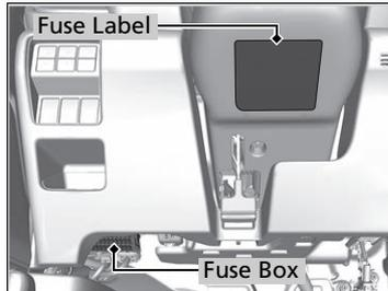
Fuse locations are shown on the label on the steering column lower cover. Locate the fuse in question by the fuse number and label number.
