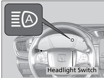
To activate the system, turn the headlight switch to **AUTO** and then set the headlights to low beam. The auto high-beam indicator will come on.
