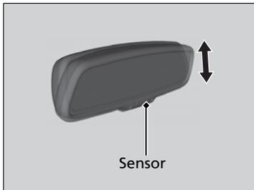
When driving after dark, the automatic dimming rearview mirror reduces the glare from headlights behind you. This feature is always active.
