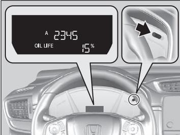
1. Turn the ignition switch to ON **II** and have the vehicle at a complete stop.
