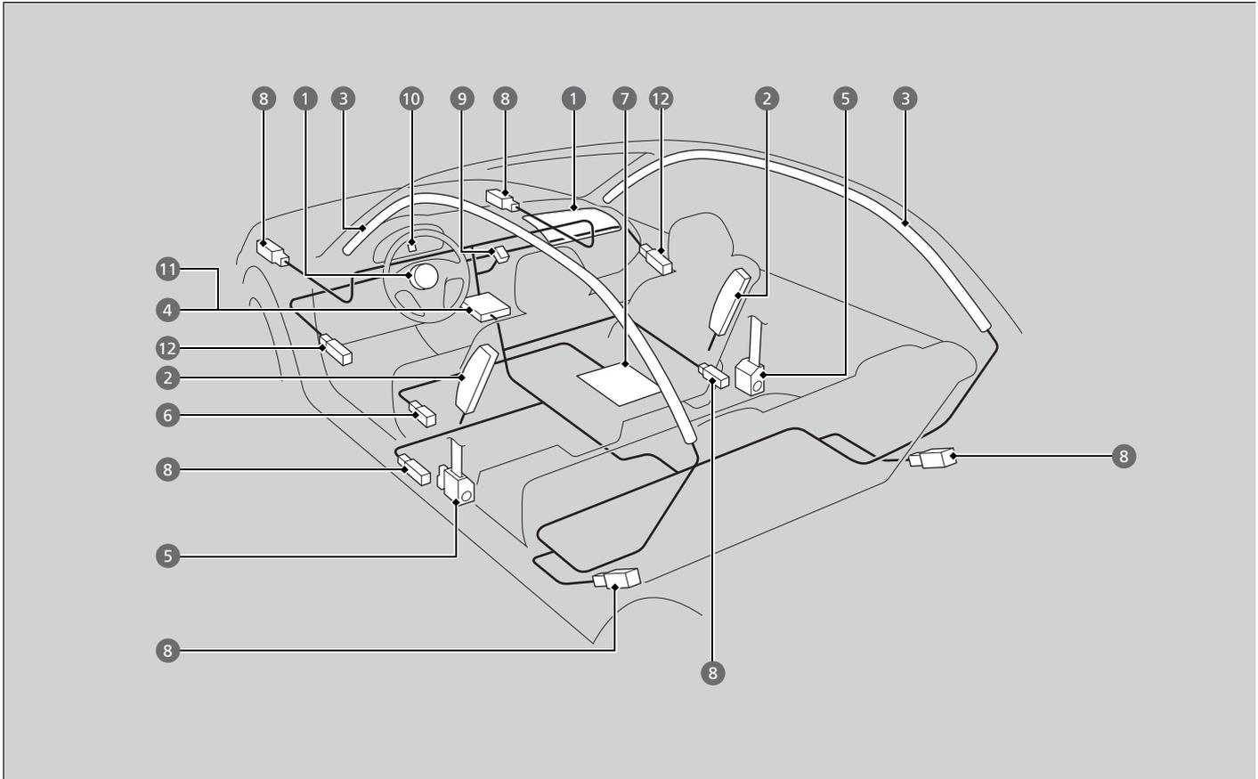
The front, front side, and side curtain airbags are deployed according to the direction and severity of impact. Both side curtain airbags are deployed in a rollover. The airbag system includes:
