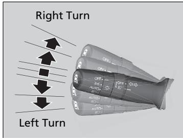
The turn signals can be used when the ignition switch is in ON
