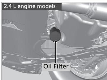
5. Remove the oil filter and dispose of the remaining oil.
