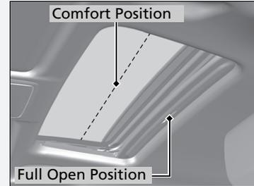
The panoramic roof cannot be fully opened in a single operation. The panoramic roof has a "comfort" position or wind noise reduction position at which the roof first stops. To open fully, pull the switch back again after the roof has stopped at this position.
