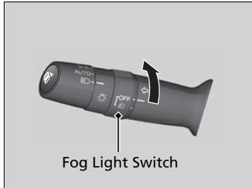
Can be used when the low beam headlights are on.
