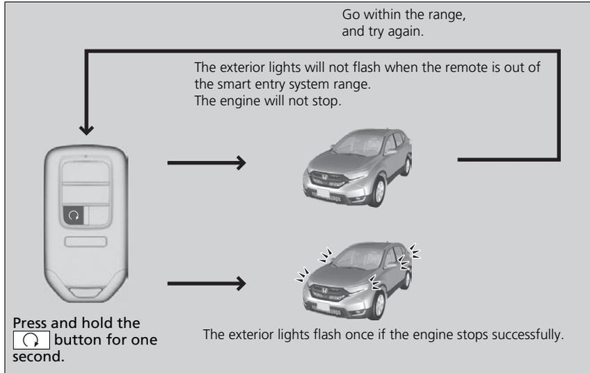
⊞ Remote Engine Start with Vehicle Feedback\*
