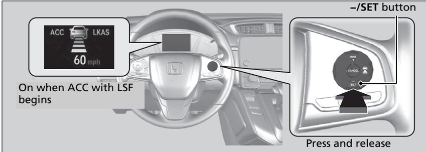
**When driving at 25 mph (40 km/h) or above:** Take your foot off the pedal and press the **-/SET** button when you reach the desired speed. The moment you release the button, the set speed is fixed, and ACC with LSF begins.
