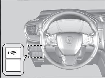
Press the heated windshield button to deice the windshield when the power mode is in ON.
