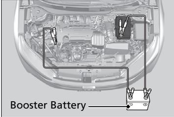
5. Connect the other end of the second jumper cable to the engine hanger (as shown). Do not connect this jumper cable to any other part.
