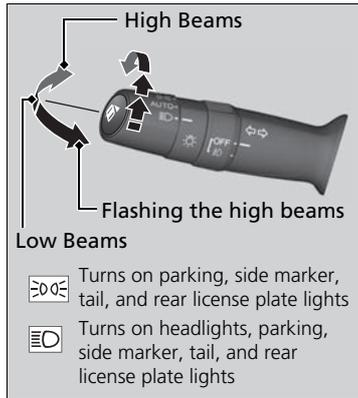
Rotating the light switch turns the lights on and off, regardless of the power mode setting or position of the ignition switch.
