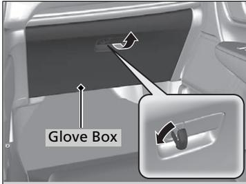
Pull the handle to open the glove box. You can lock the glove box with the master key or the built-in key.
