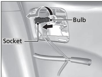
3. Turn the socket to the left and remove it. Remove the old bulb.
