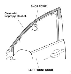
5. Peel back approximately 1½ to 2 inches of adhesive backing from each adhesive tape, and tape the ends to the front surface of the left front door visor with masking tape.
