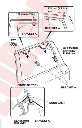
13. Install two brackets A between the door sash and the glass run channel at the measurements shown. Seat the glass run channel properly around the brackets.
