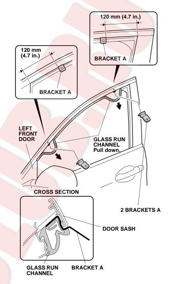
Install two brackets A between the door sash and the glass run channel at the measurements shown. Seat the glass run channel properly around the brackets. 4. Using isopropyl alcohol on a shop towel, thoroughly clean the door sash where the left front door visor will attach.
