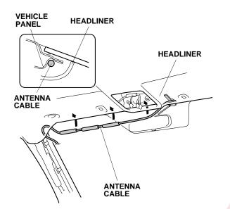
34. Using isopropyl alcohol on a shop towel, thoroughly clean the vehicle panel, where the urethane tapes will attach.
