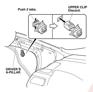
12. Temporarily reinstall the driver's A-pillar trim, and check the overlap between the headliner and the driver's A-pillar trim according to the service manual. Remove the driver's A-pillar trim. Install the new clip (supplied) to the driver's A-pillar trim.
