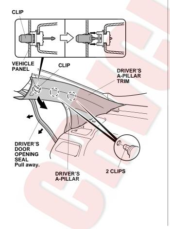
9. To prevent the clips from falling into the vehicle body, roll up the shop towel, and insert it between the driver's A-pillar and the dashboard. Take care not to damage the driver's A-pillar.
