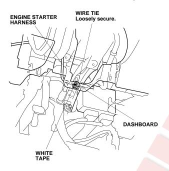
71. Route the engine starter harness up steering wheel as shown.
