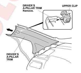
11. Remove the remaining upper clip from the driver's A-pillar.
