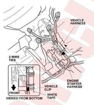
72. Align the white tape on the engine starter harness with the vehicle clip, and secure the engine starter harness to the vehicle harness with two wire ties as shown.
