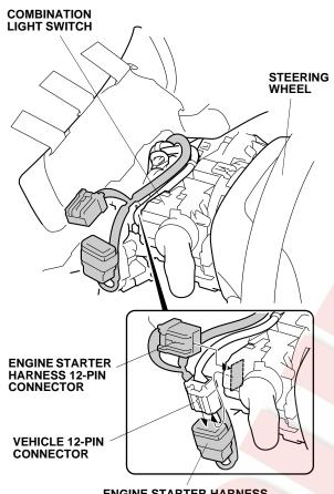
ENGINE STARTER HARNESS 12-PIN CONNECTOR
