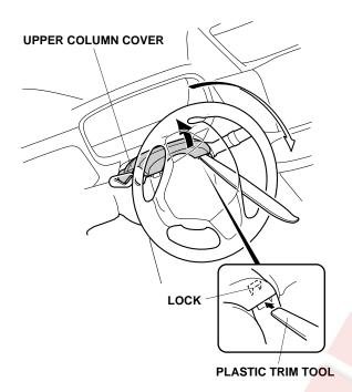
21. Secure the upper column cover to the meter panel with the tape.
