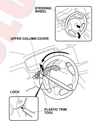
19. Using a plastic trim tool, release the lock as shown.
