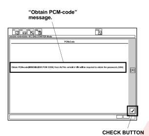
Input the PCM Code, then click the check button. NOTE: To ensure security, the PCM code (password) is changed everyday, so it is impossible to register the remote control engine starter if the dates of the PCM code acquisition and registration are different. The date of the HDS tester should also
