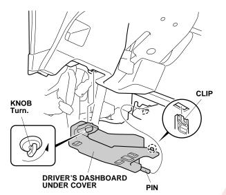
16. Remove the driver's dashboard lower cover (eight clips and unplug the vehicle connector).
